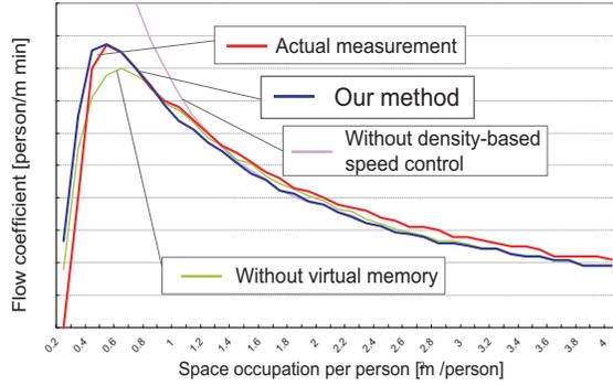
Figure 9: Comparison of flow coefficient with actual measurement
