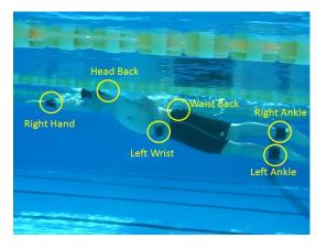
Fig. 3. Attached locations of 6 sensors.
